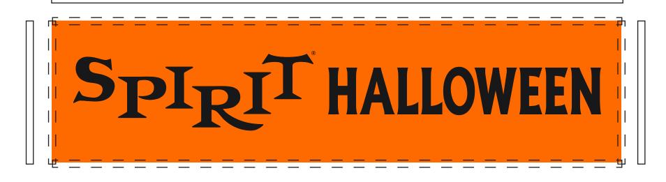
2" Clear Vinyl strips are used as adhesive to hold graphic in place. Dotted lines represent where the clear vinyl adhesive would go.
